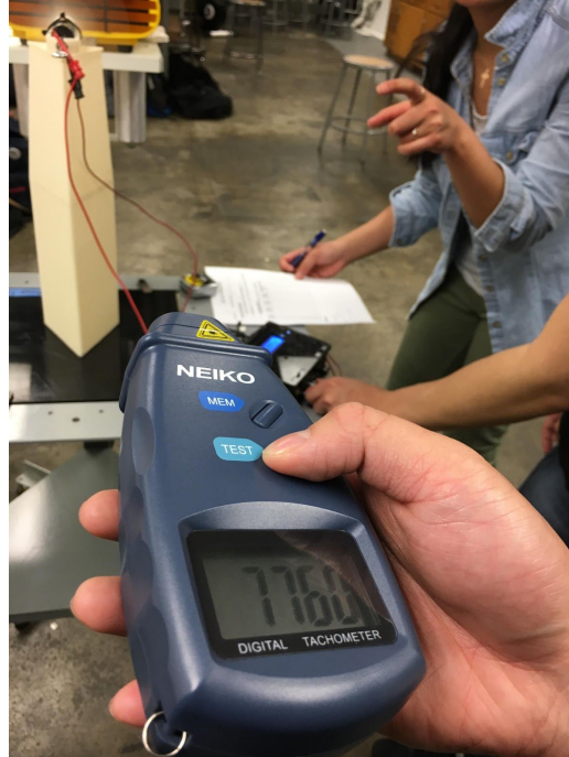
Figure 10: We also used a tachometer (shown above) to measure the speed in rpm of the blade. To use the tachometer, we attached a piece of reflective tape to the blade. The tachometer has a laser which uses the reflective tape to generate a reading of the blade speed.
