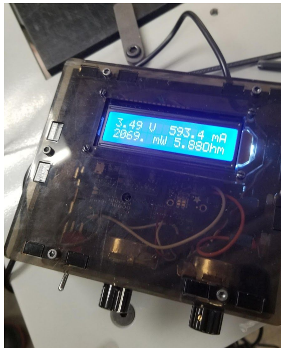
Figure 11: Finally, we used an electrical meter to measure voltage, current, and power and a load box to draw power. The load box has a potentiometer which controls how much power is drawn. The electrical meter and load box were located in one device (shown above).
